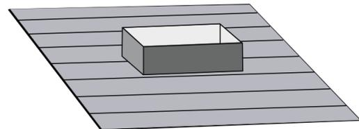
Loosen the combi brackets and mount the roof led thru in the frame from above. Seal the frame requisitely. If necessary, also seal between frame and roof led thru.
