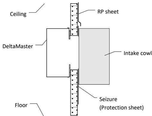
In order to prevent fiber release from wall insulation, a wall led thru should be mounted in the wall. Install from the inside of the wall.
