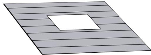
Make a frame of plywood or similar around the hole in the roof. Adjust the height of the frame to the length of the roof led thru (Recommended min. length is 500 mm to reduce risk of snowmelt).
