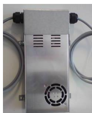
Power converter 230V/48V
