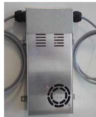
Power converter 230V/48V
