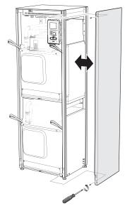
The side covers can be removed to facilitate the installation.
