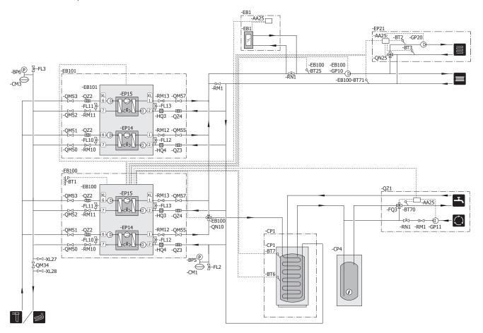
The heat pump (EB100) prioritises charging of hot water with a cooling module (EP14) via a reversing valve (EB100-QN10). When the water heater/accumulator tank (CP1) is fully charged, (EB100-QN10) switches to the heating circuit. When there is a demand for heat, cooling module (EP15) starts in heat pump (EB101) first. In the event of a large demand, cooling module (EP14) also starts in (EB101) for heating operation.
