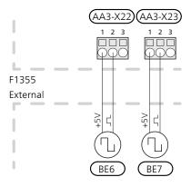
Activate the energy meter(s) in menu 5.2.4 and then set the desired value (energy per pulse) in menu 5.3.21.
