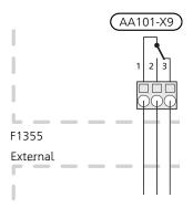
The picture shows the relay in the alarm position.
