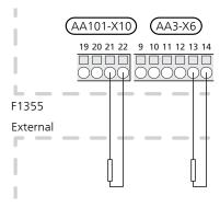
The example above uses the inputs AUX3 (AA3-X6:13-14) and AUX5 (AA101-X10:21-22) on the terminal block.
